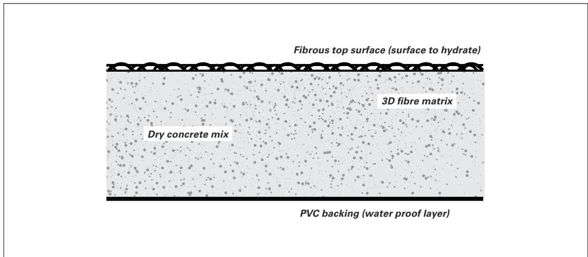
FIG. 3 Cross section
