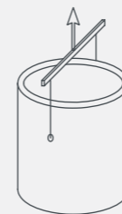
Concrete Manhole 2-point lift using lifting beam
