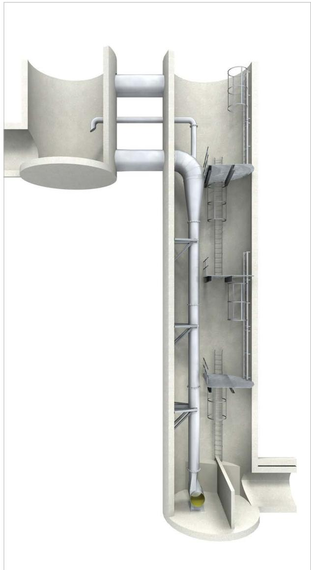
FIG. 1 Drop Shaft with access
