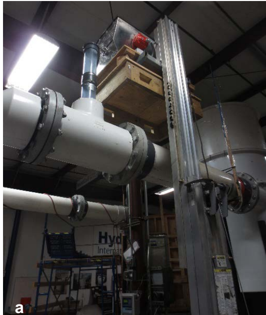
Figure 5 a) Influent Feed Port for Removal Efficiency Testing, b) False Bottom Locations
