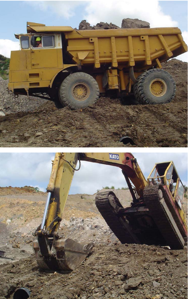
FIG. 1 Laylite Culvert withstanding weight of various heavy vehicles
