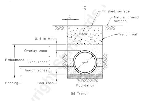
FIGURE 1 FILL AND PIPE SUPPORT TERMS
