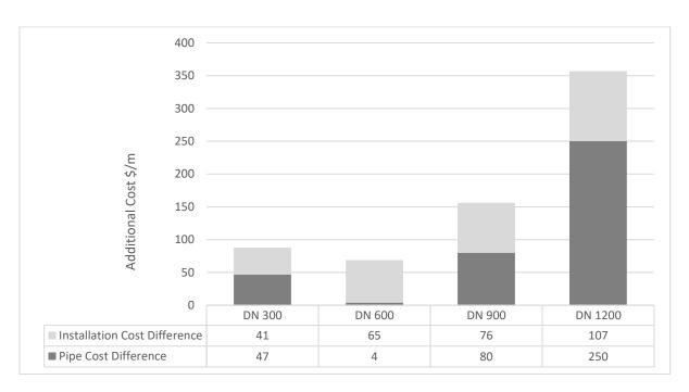
Figure 1 Makeup of Additional Cost of GRP over Concrete Pipe Installations
