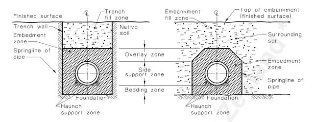
FIGURE 1.1 BURIED FLEXIBLE PIPE INSTALLATION—TERMINOLOGY
