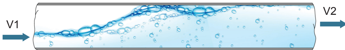
Fig. 37 Air pockets inside the pipe
