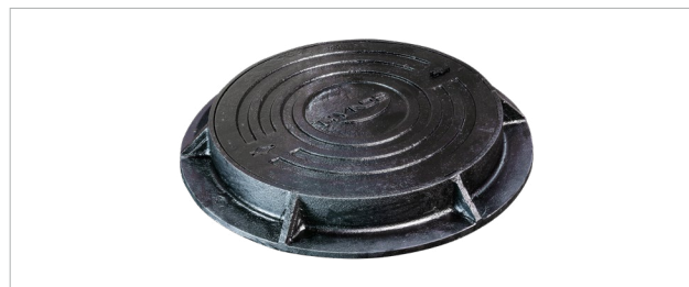
FIG. 6 Cast Iron Cover and Frame Ø540 mm rated to 80kN
