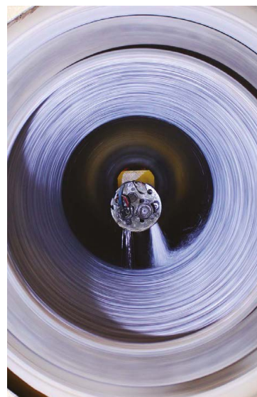
FIG. 6 Centrifugal Casting (CC) manufacturing process.
