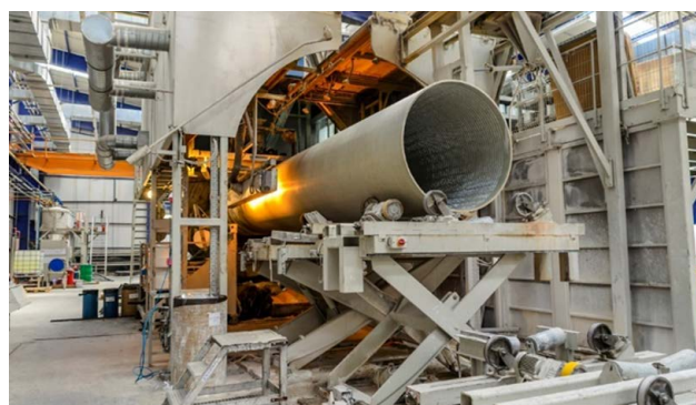
FIG. 4 Continuous Filament Winding (CFW) pipe manufacturing process
