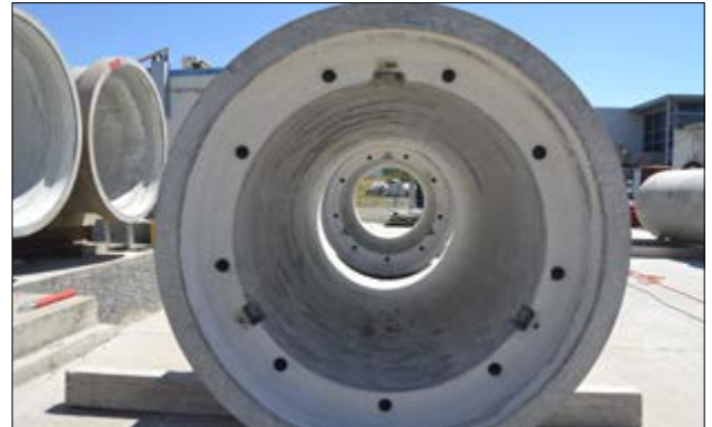
FIG. 3 Pipe with seismic mushroom fitted to collar back wall.
