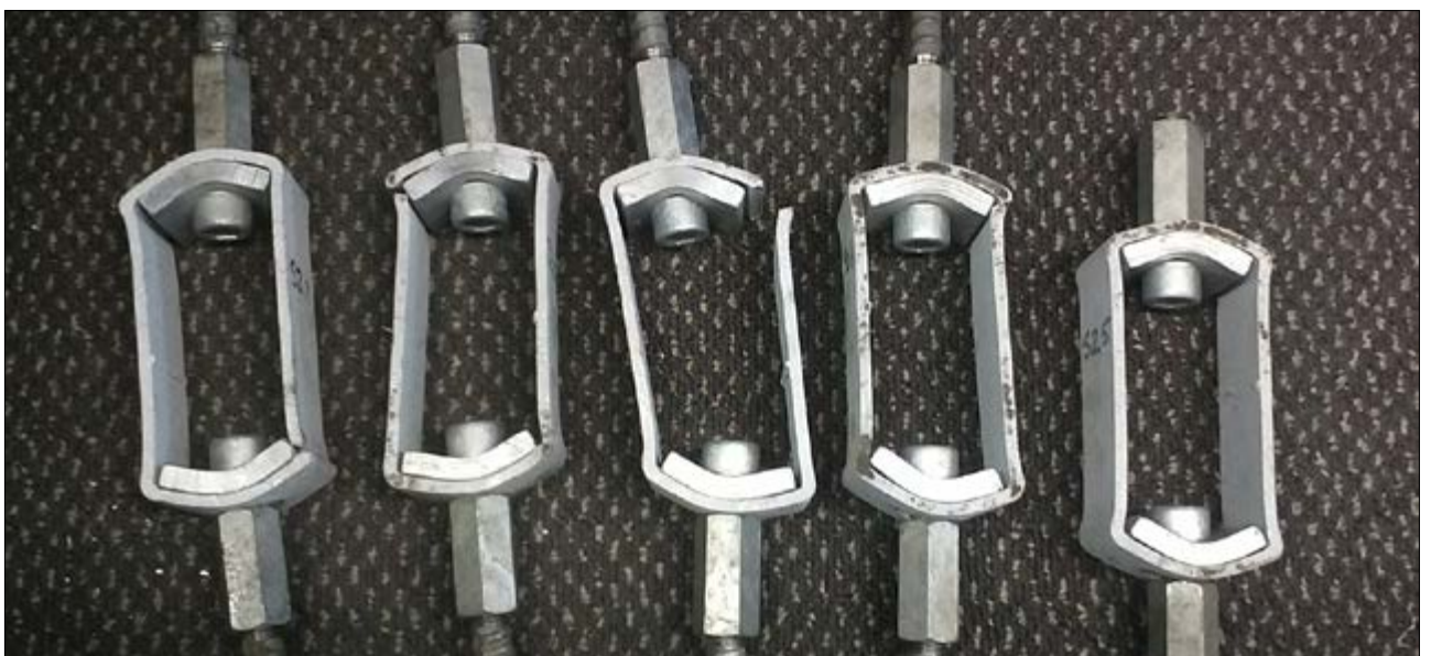
FIG. 8 Restraint assemblies after testing to breaking load
