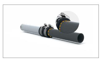
4. Position the remaining pipe, ensuring the coupling face and marked line are flush. Tighten this clamp band.
