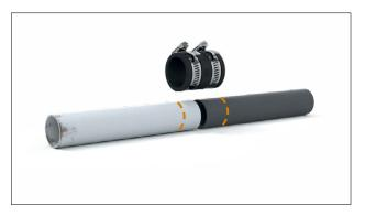
1. Mark both pipes, from the end to be connected, half the width of the coupling, less the required joint gap, which is usually 10mm
