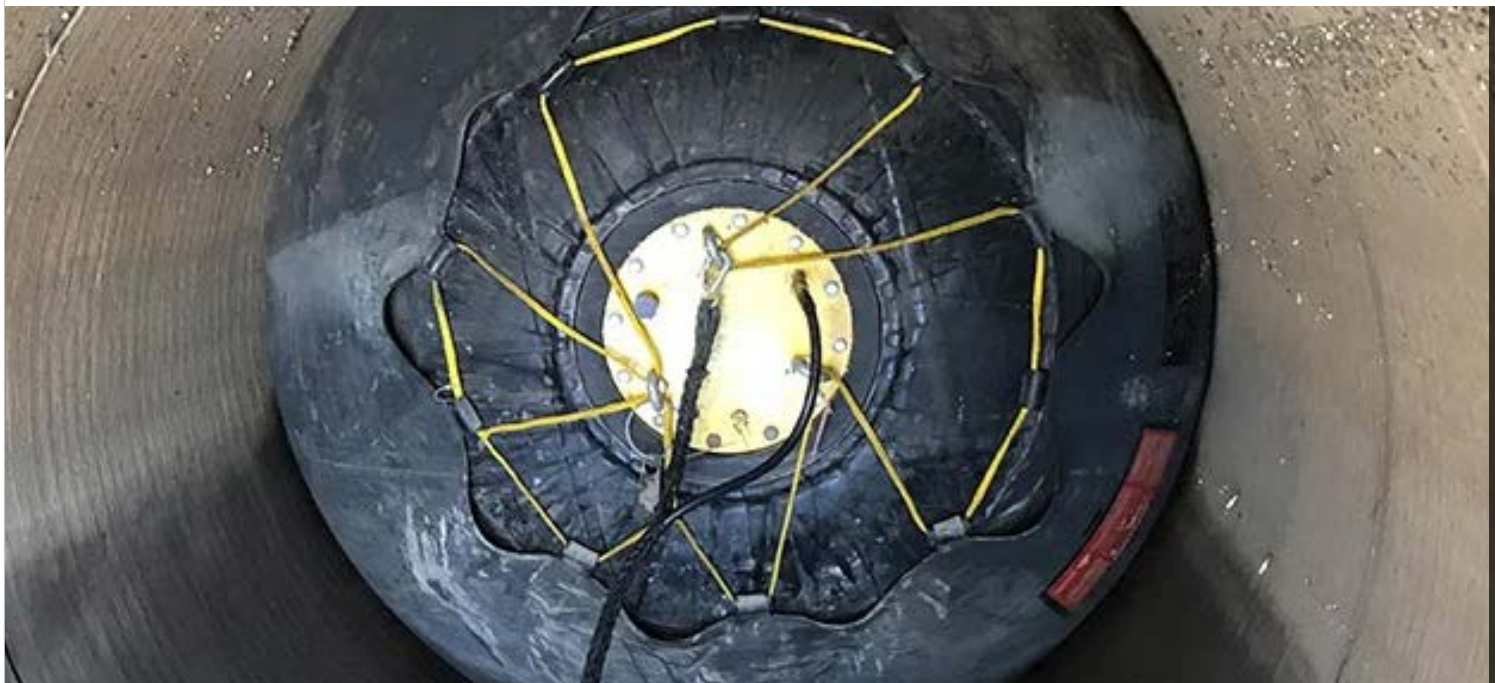
01.24 | DRAINAGE | D10.13 PNEUMATIC PIPE PLUGS
