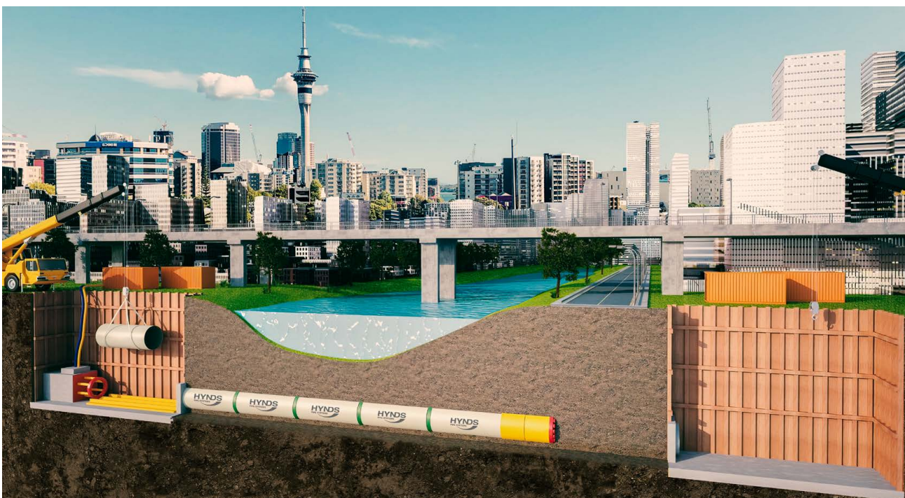
FIG. 2 Typical example of Micro Tunnelling operation illustrating launch shaft, hydraulic jack, concrete jacking pipes, tunnel boring machine (TBM) and retrieval shaft.
