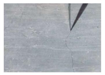
Cracks in concrete pipe under external load. Feeler gauge is used to test crack width
