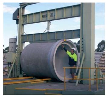
Load testing of Steel Reinforced Concrete Pipe
