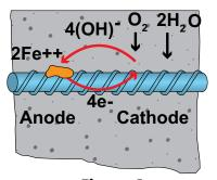
Figure 1 Simplified model of corrosion process
