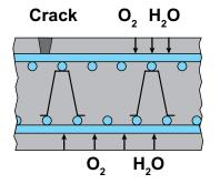
Rate of corrosion =  $f(O_2, H_2O$  at Cathode) (Resistivity of Concrete)(Size of Cathode)
