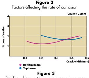
Reinforced concrete in a marine environment -Loss of section of reinforcing bar
