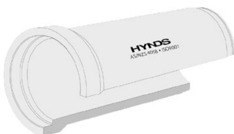
FIG. 1 Schematic elevation/cross section of Hyspec Spun Concrete Rubber Ring Joint Pipe
